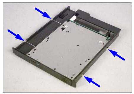
Figure 17: Mounting the drive in its frame
